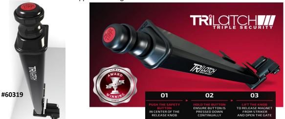
**Safe Tech SL50 TRI** Gate Latch uses a unique dual action to operate the latch. In order to open the gate, the button on the lever must be depressed. Adjustable, both vertically and horizontally. Lockable with and without keys. Stainless Steel components and a Fiber Reinforced Polymer Bind-Free Operation. UV Stabilized and Rust Proof. Approx. 21" long.
